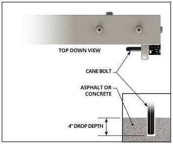
**10.** Minimum depth of receiver hole is 4" at the Closed and Open position of the door. *Failure to comply with this will result in a voided warranty.*
