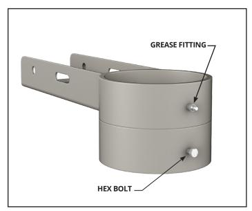
Apply grease with a grease gun at the GREASE FITTING on the HINGE RING SADDLE BRACKET.
