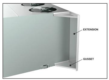
**1.** If any **EXTENSIONS** or **GUSSETS** are required, install them per the submittal drawings supplied with the kit. Be sure to install these components in the proper locations before attaching the **CORNER TRUSSES**.
