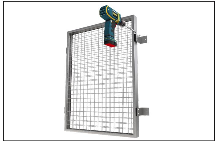
3. Once you have all **BRACKETS** mounted to the frame, transfer the locations for the top of the **KEYWAY** to the mounting surface.
